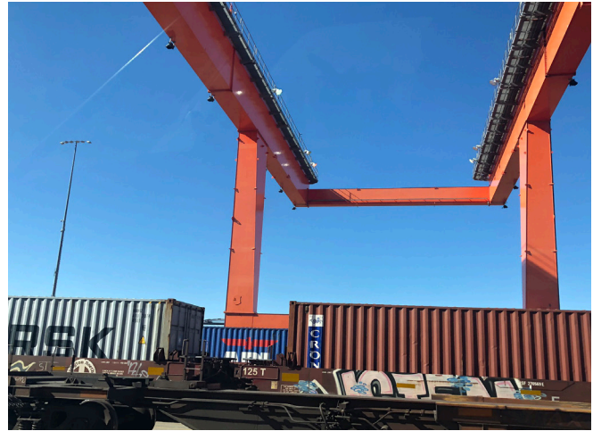
This is the view on the tracks & under the Intermodal cranes, where shipping containers get loaded/unloaded, scanned and logged before going to their next destination.
